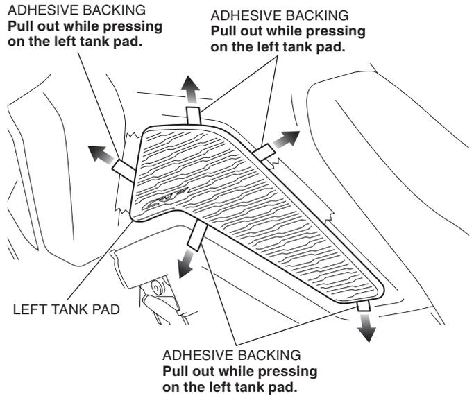
6. Remove the masking tape and apply adequate pressure to the attached left tank pad.
