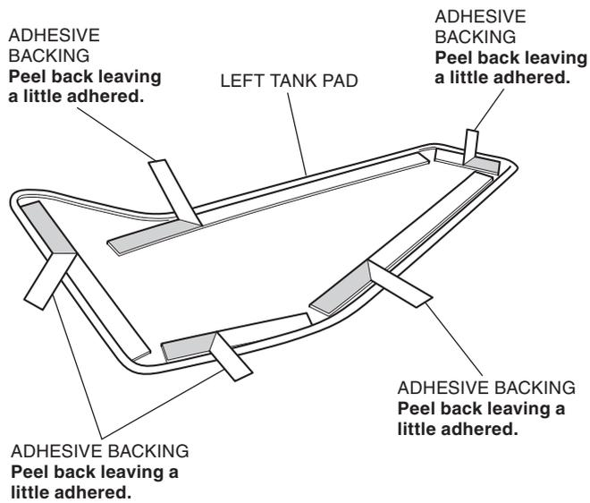
4. Attach the left tank pad as shown.
