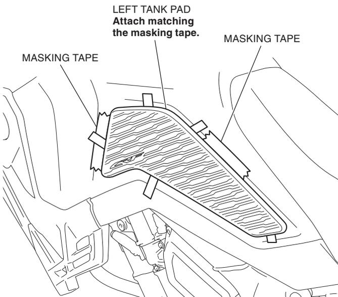
5. Remove the adhesive backing as shown.
