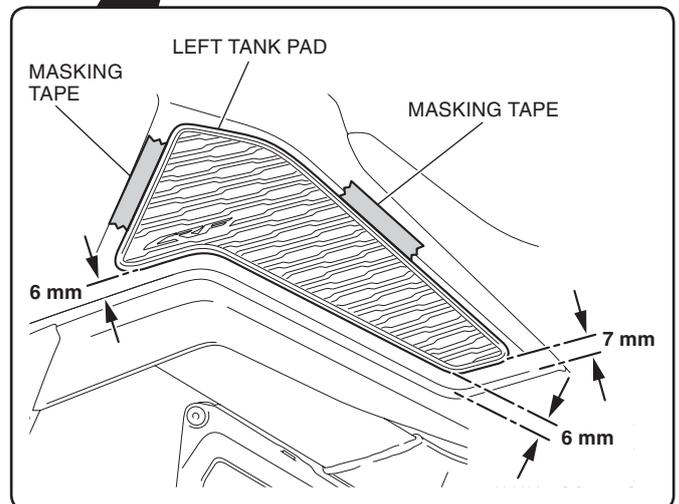
3. Peel off the adhesive backing on the left tank pad as shown.
